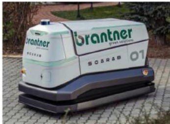
■ A cover designed by the University of Art and Design Linz makes the autonomous mobile robot SCARAB suitable for all-weather use.
