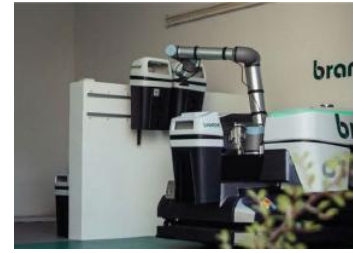
■ At the base, the containers are emptied, cleaned and checked while the robot recharges its battery.
