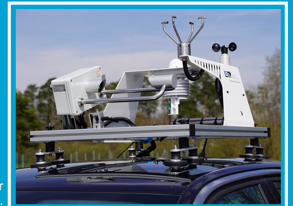
Mobile measurement scenario: weather sensors mounted on the roof of a car.
