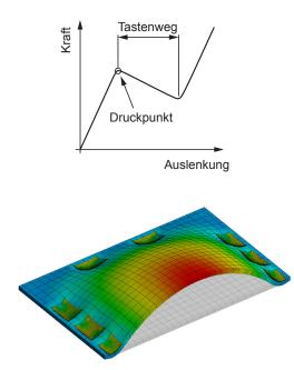
The sensor technology is based on a measurement of the deflection of the plate at different locations. This way, both the position and the intensity of the contact can be detected. When a minimum load is exceeded, the board deflects suddenly. This briefly results in a negative stiffness (a characteristic of a key confirmation) in the load deflection curve, see diagram on the left.
