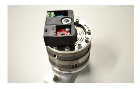
The active vibration damper is held in its zero position by a mechanical spring and deflected from this position electromagnetically. This design allows the actuator to be used in any position and cover a wide frequency range. The combination of permanent and electromagnets and the optimised ratios of the mechanical and electromagnetic factors make it possible to achieve high performance with small size and low weight.
