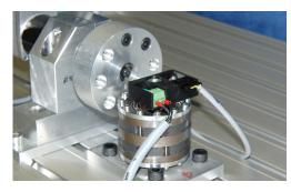
Thanks to its robust and easy operation, the active electromagnetic vibration damper can be used in practically any situation where there is sufficient space for installation. Examples include:
